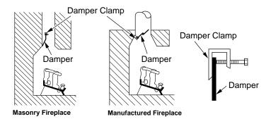
Figure 10 - Attaching Damper Clamp
